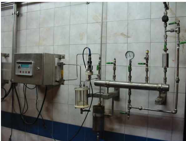
Fig. 3 CO 2 sampling for flow cell 32001.XXX and EC sensor
