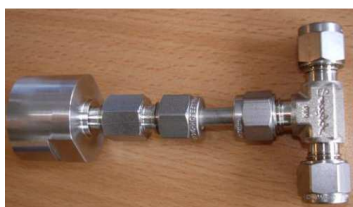
Fig. 7 Adapter 33058 with flow chamber for pressure sensor
